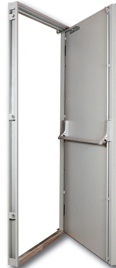
Door leaf prepared with threaded nutserts located to accept Exidor 294 panic bolt (panic bolt supplied loose complete with shoot tubes cut to size).
